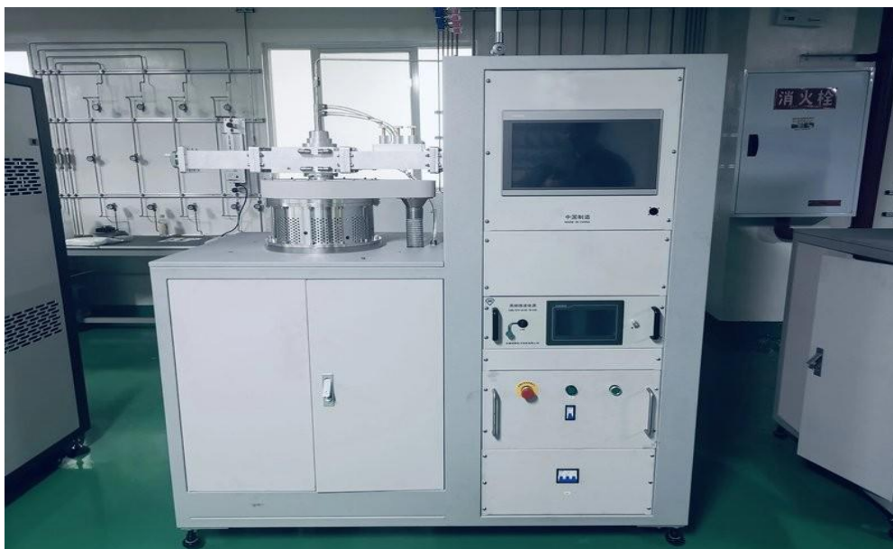
Figure 2. An example of industrial Hot-Wire CVD diamond coating equipment.
